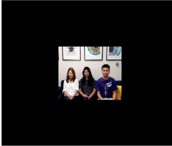
This mode allows you to change the Field of View (FOV) of the screen. This helps individuals with Retinitis Pigmentosa or Glaucoma to be able to see better by shrinking the entire image into a smaller viewing area.
